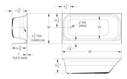
**General:** Furnish and install as shown on plans, TOPAZ® bathtub as manufactured by E.L. Mustee & Sons, Inc. Shall be a fiberglass 30" x 60": right hand or left hand Model \_\_\_\_\_\_. Construction shall be molded, reinforced fiberglass using matched metal molds under extreme heat and pressure. Shall meet ANSI Specification Z 124-2017. Color: \_\_\_\_\_\_ (White, Bone, Biscuit) Weight: 55 lbs. Install in compliance with local codes.
